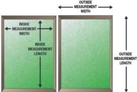
drop, add 100-150mm on top and 30-50mm on bottom to window outside measurement.
